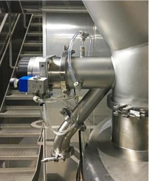
The sampling valve allows the operator to extract a sample of the product from the production line or reactor and safely store it for transportation to the laboratory where it will be analyzed or to the archive room where it can be retrieved for further use. The Gericke sampling valve is designed according to the latest construction standards and recognized safety rules.
